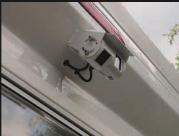
Rear camera fitted to a 2006 Marquis Lancashire (Auto-Sleeper Nuevo) coach
